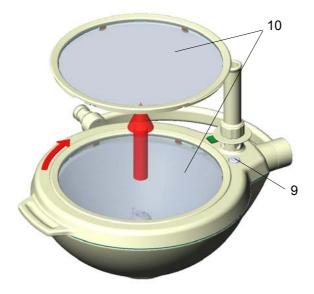
Then remove the retaining ring 10 by pulling it upwards.
