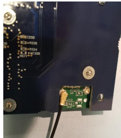
Antenna connection to WLAN module connect as shown.
