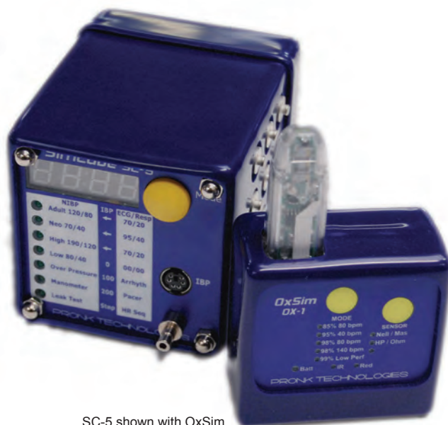
SC-5 shown with OxSim SpO2 simulator.
